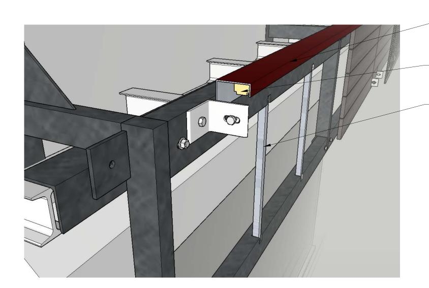
INSTALLED W/ SELF-DRILLING FLAT HEAD TORX SCREWS W/ BLACK OXIDE FIN. W/ COUNTER SINK
